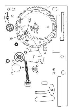
Fig.4-4 DATUM POSITION OF PINCH LEVER TOTAL ASS'Y & CAM GEAR
